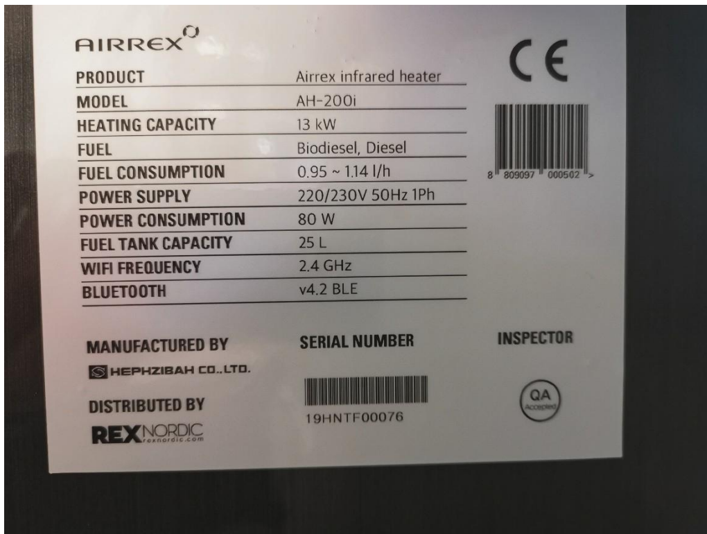
Image 2 AIRREX AH200i identification data
