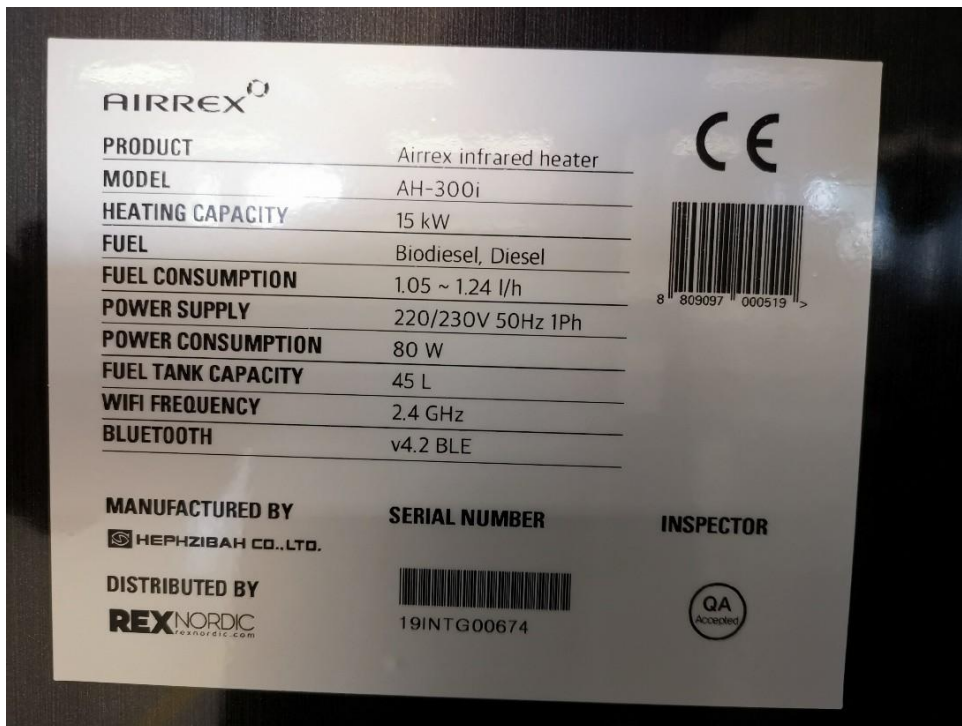
Image 4 AIRREX AH300i identification data
